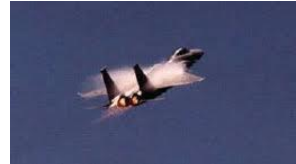
Flow Visualization of Vortex from the LEX Bursting ahead of the Vertical Tail
