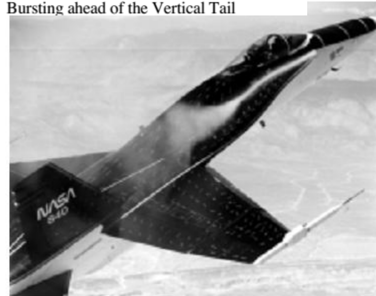
Flow Visualization of Vortex from the LEX Bursting ahead of the Vertical Tail
